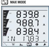
Max values for voltage, current (including neutral current), power and harmonics
