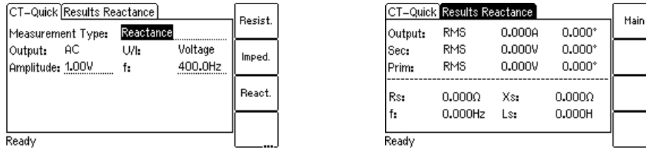
Figure 10-21: CT-Quick card and Results card for reactance measurement
