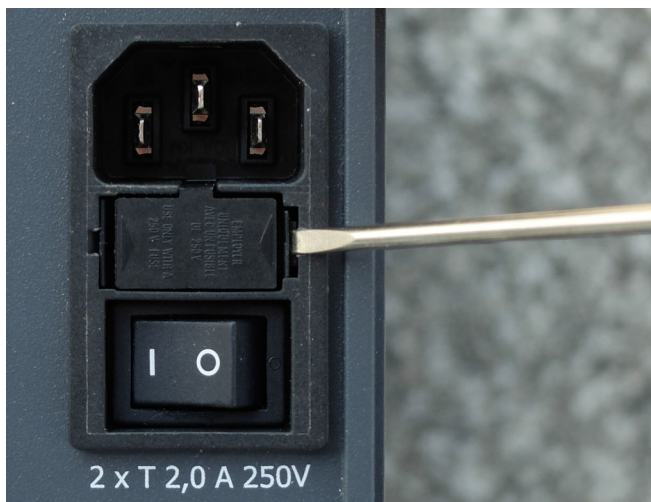
Figure 11-1: Unlocking the locking tongues of the fuse holder
