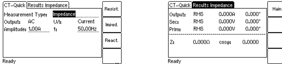
Figure 10-19: CT-Quick card and Results card for impedance measurement
