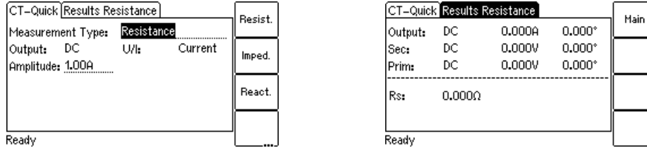
Figure 10-15: CT-Quick card and Results card for resistance measurement
