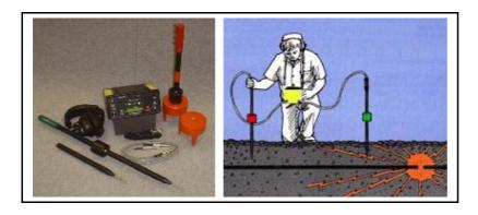
Ease and speed of fault finding with a thumper have been greatly enhanced with the addition of the S.D.A.D. to the Aqua-Tronics line. The Super DAD conveys more information about the fault location, and faster, with the addition of new microprocessor controlled electronics that provide bright, easier-to-see-and-read signals - day or night.
