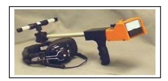
This is a low-cost receiver that is tuned to 50-60 Hz and picks up the electromagnetic wave when current is present in the cable. It will detect loaded lines where most others fail, because of advanced receiver circuitry and a precision wound antenna.
