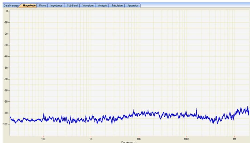
**Figure 3.17 Open-Circuit Lead Response**
