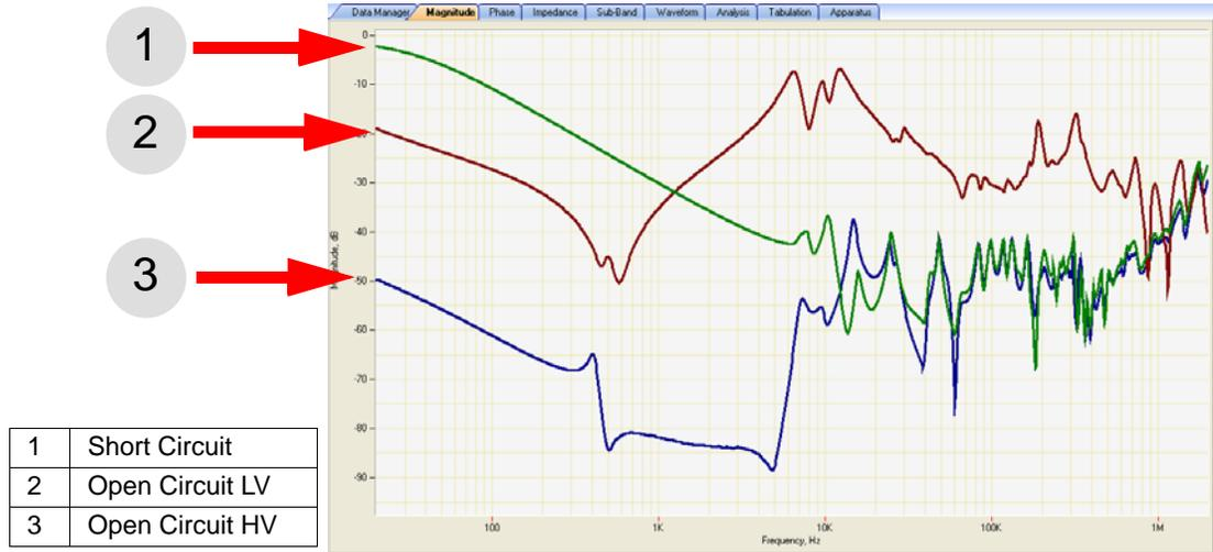
**Figure 3.40 Responses for One Phase of a Transformer HV Delta Trace**
