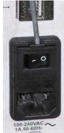
*Figure D.2 Blade in Top of Fuse Cover*
