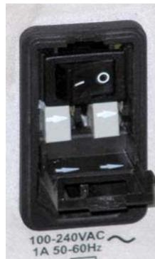
*Figure D.3 Open Fuse Cover with Fuses in Place*
