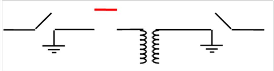
Figure 3.20 Removed Isophase or GIS Link
