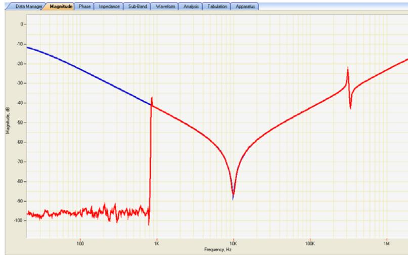
*Figure 3.39 Typical Open-Circuit Trace*
