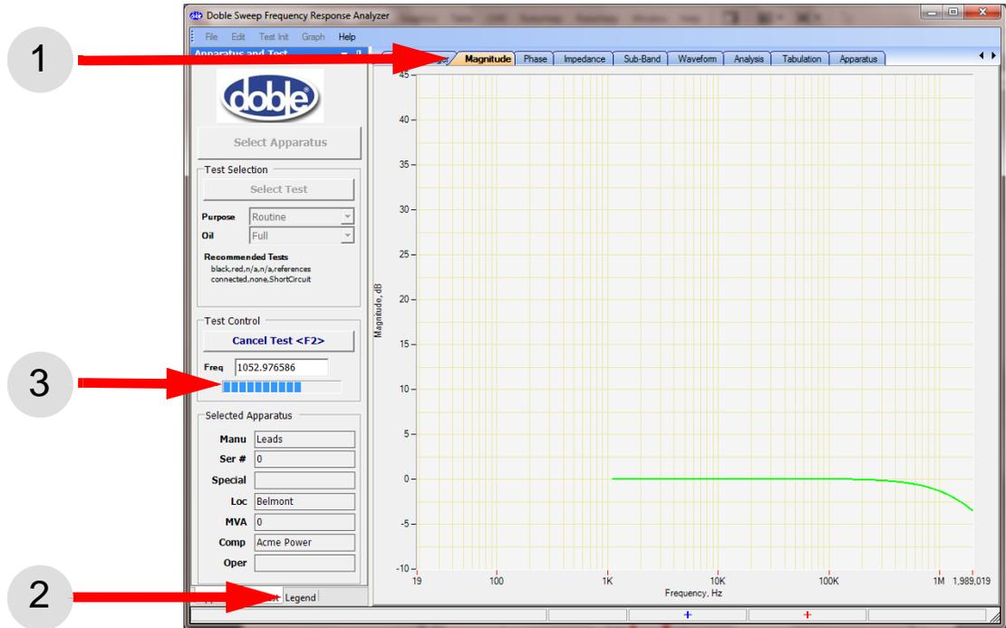
Figure 3.15 Shorted-lead Test in Progress
