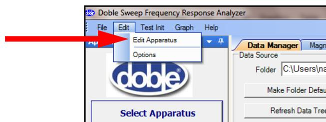
*Figure 3.24 Edit Apparatus Option on Edit Menu*
