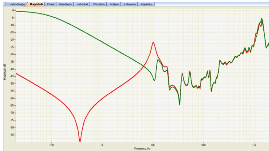
Figure 3.46 Shorted Turn on One Winding
