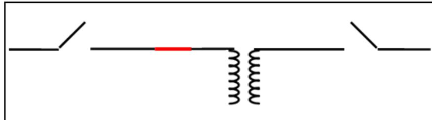
*Figure 3.18 De-energized and Disconnected Transformer*
