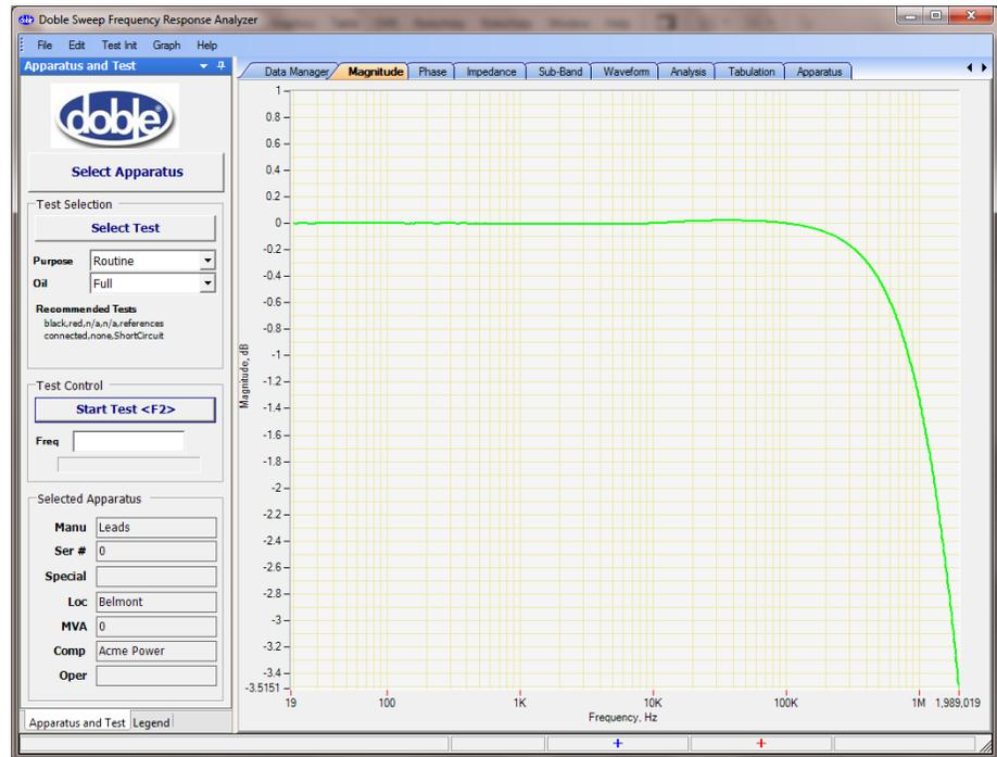
**Figure 3.16 Correct Shorted-lead Response**
