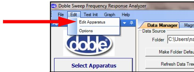
*Figure 3.5 Edit Apparatus Option on Edit Menu*
