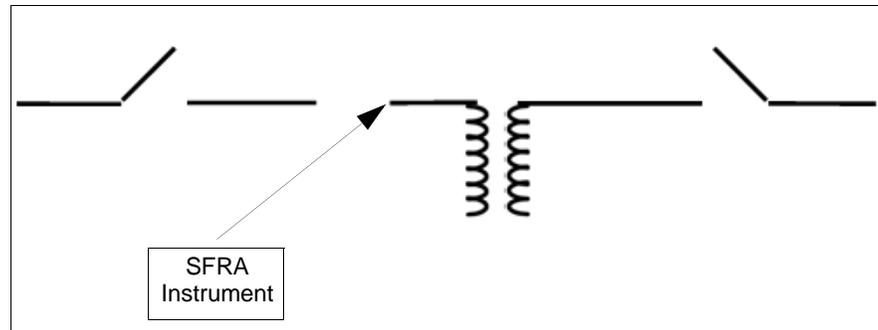
*Figure 3.23 Removed Temporary Static-Discharge Grounds*
