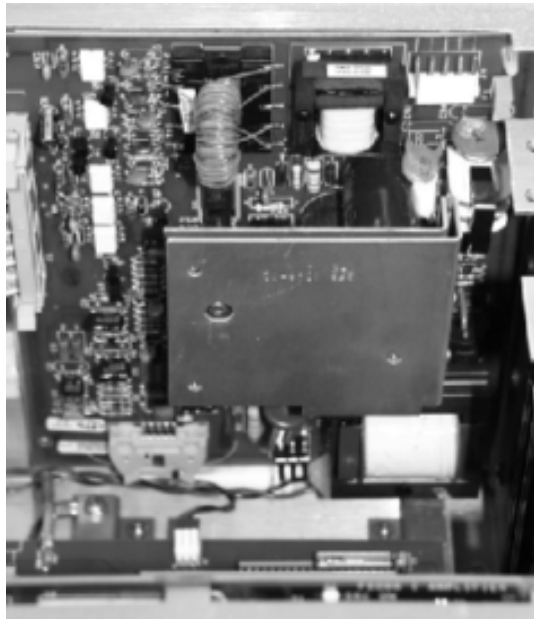
Figure 5-18 Fixed Output Battery Simulator Mounted at the Back of the Instrument
