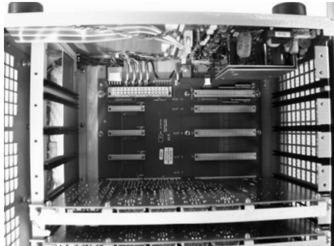
Figure 5-19 Remove Power Supply and Voltage Amplifiers to Access Battery Simulator
