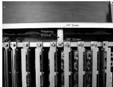
Figure 5.11 Retaining Bracket for Cooling Fan Assembly
