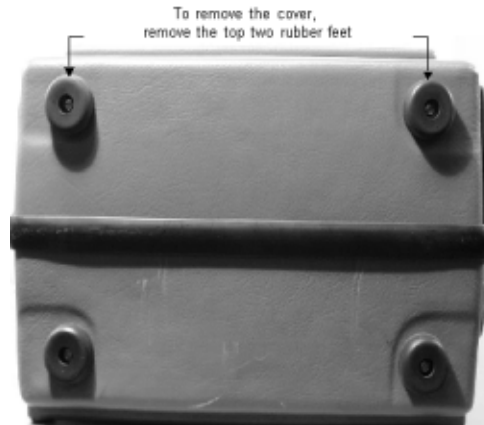
Figure 5.2 Remove Rubber Feet
