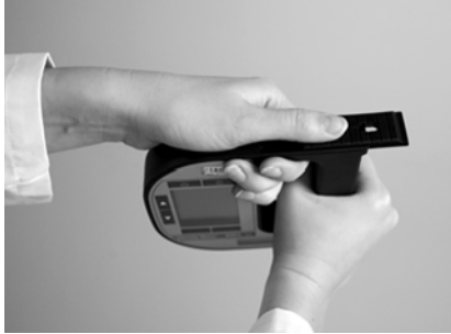
Fig. 12 - 3 Removing the pump lock
