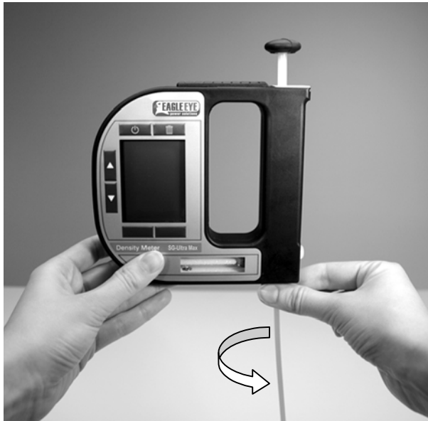
Fig. 7 - 1 Connecting the filling tube
