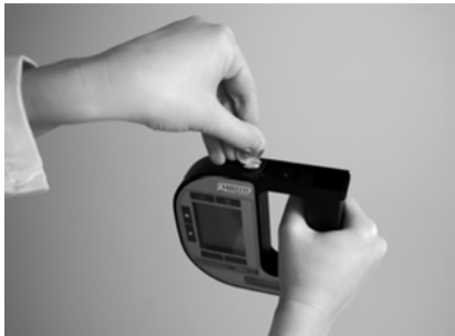
Fig. 12 - 4 Opening the battery cover
