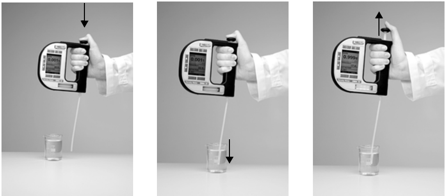
Fig. 10 - 1 Filling sample using the filling tube
