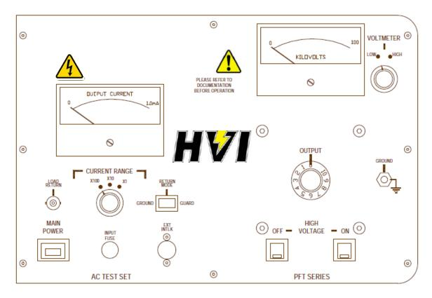
Figure 1B PFT ANALOG Series front panel controls.
