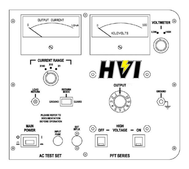
Figure 1C PFT-652/1003 Series front panel controls (Two Piece).
