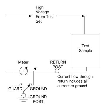
Figure 2, Grounded Return Diagram
