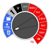
There are two delete functions; delete a single result and delete all results. Select the bin icon on the central rotary switch. The first record indicated contains the result of the last test performed. Up / down arrows navigate through records and the OK button is used to select delete where the 'X' changes to a tick and the on screen bin icon flashes. A subsequent press of the OK button activates the deletion.
