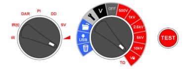
Instrument controls are simple to operate. The central rotary switch incorporates the OFF position. The left hand rotary switch selects insulation test type (test mode switch). The TEST button starts and stops a test.
