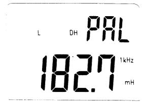
2) Similarly, to get the series mode data either under the Capacitance or Resistance measurement, press the DH key and then press and hold D/Q button for one second. When the " [[] " character appears on the secondary display, the main digital reading displayed will be the series mode data. Press D/Q button again to exit.
