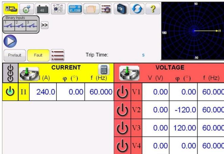
Figure 320 Manual Test Screen – Single Phase Operation
