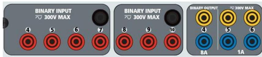
Figure 272 Binary Inputs 4 to 10 and Binary Outputs 4 to 6
