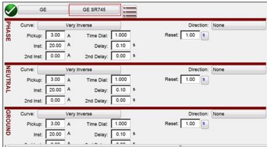
Figure 62 Curve Button location (Red boxed) in Nameplate Configuration Screen
