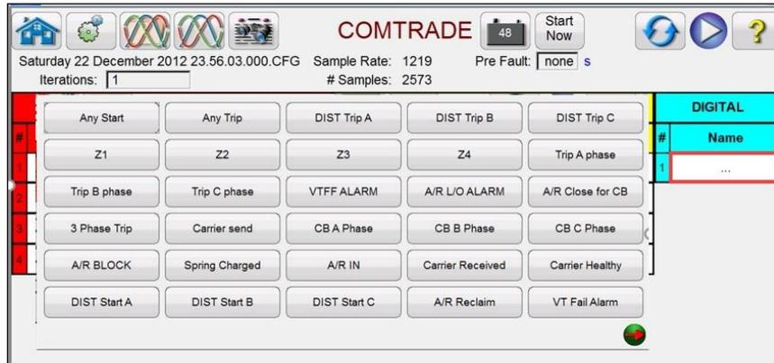
Figure 156 Selecting Digital Channels for Playback
