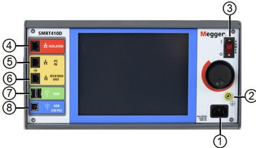
Figure 313 SMRT410D Front Panel
