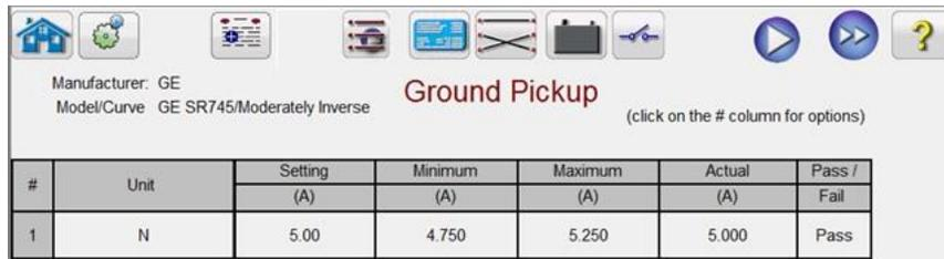
Figure 83 Example Ground Pickup Test
