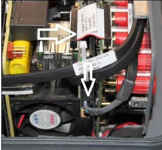
Figure 311 VIGEN1 to Front Panel Cable
