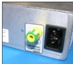
Figure 213 SMRT1 Rack Mount Back Panel Power Input
