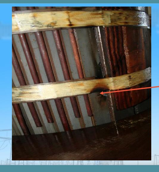
Burnt insulation may be due to PD shorts the Flitch plate to the C phase core
