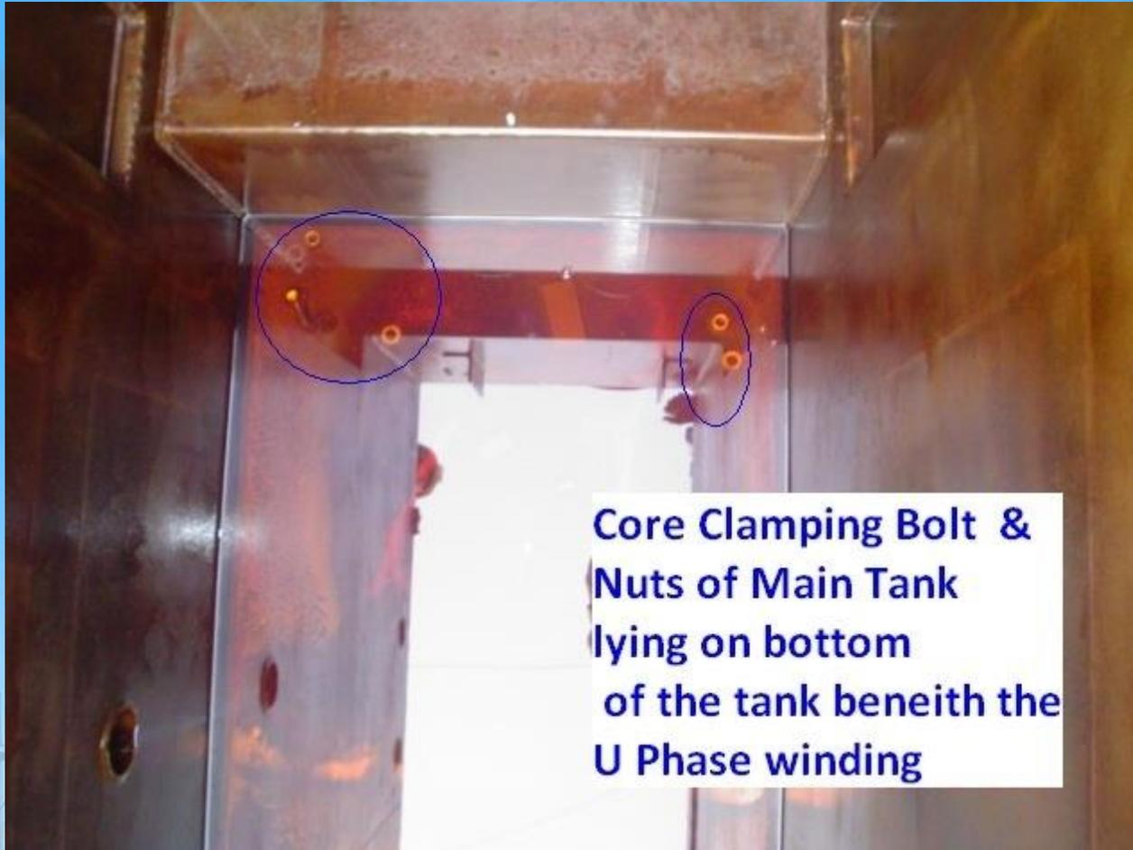
**Core Clamping Bolt & Nuts of Main Tank lying on bottom of the tank beneath the U Phase winding**
