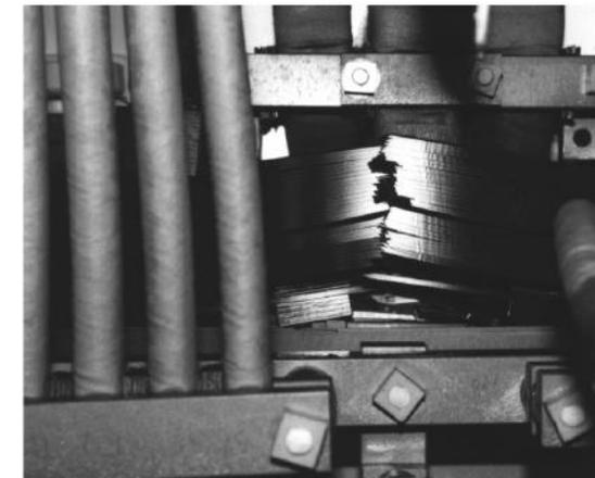
End winding support collapse
