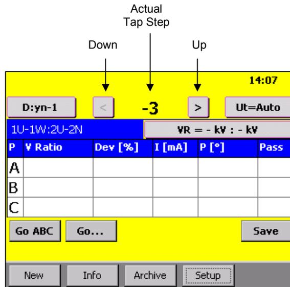
You may wish to know what for instance “tap 5” means in volts. Or you would like to switch to the 22kV Tap. Both can be done easily by touching the ‘Actual Tap Step Number’ (-3).
