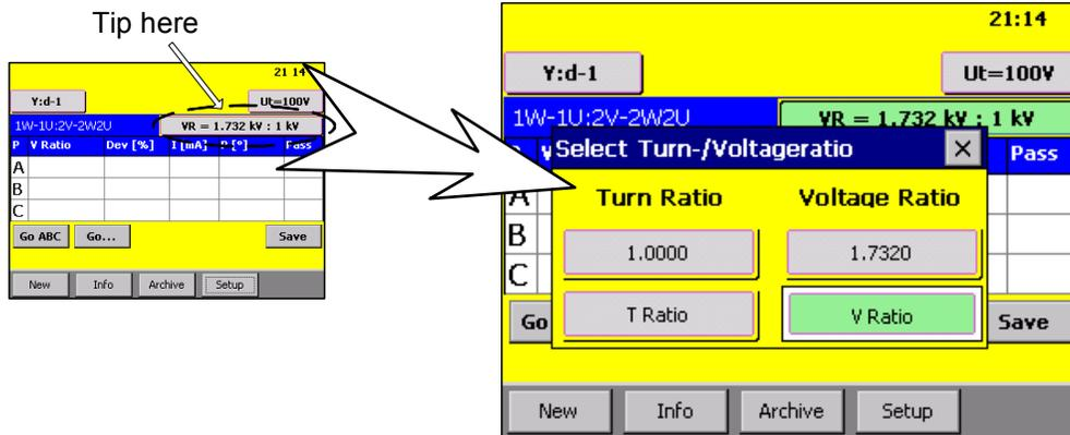
To simplify your work, we provide up to four display options for the entered transformer data. The buttons 'T Ratio' and 'V Ratio' will lead to a non calculated view. That means that you will get for instance nominal voltages instead of a calculated ratio displayed. The buttons with a number will directly display the calculated nominal ratio, based on data in the info field.
