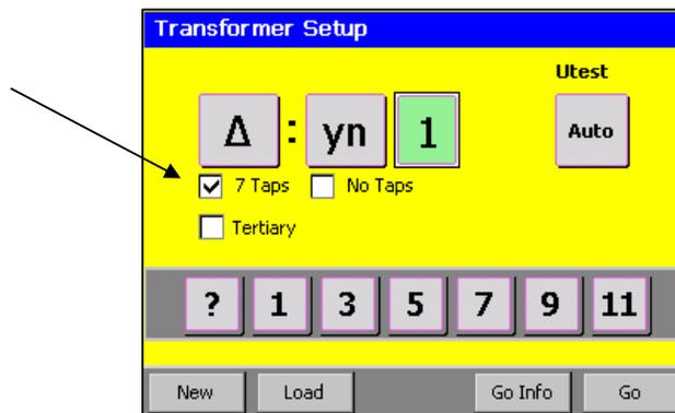
Your Transformer may have taps on the primary and on the secondary winding system. Use the same procedure to define the secondary taps.
