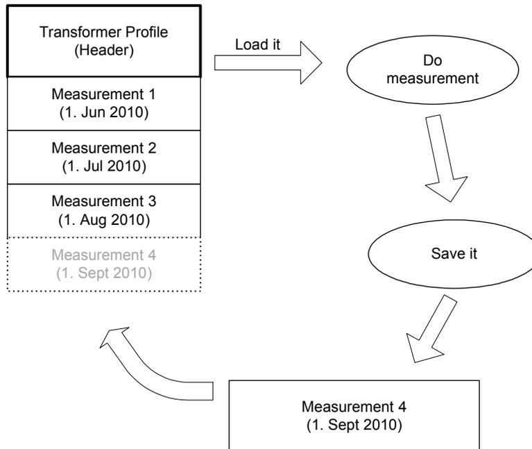
This shows a Transformer that has been created and measured for the first time on Jun 1<sup>th</sup> 2010. Profile and Measurement was saved by touching the 'save' button in Main Screen.
