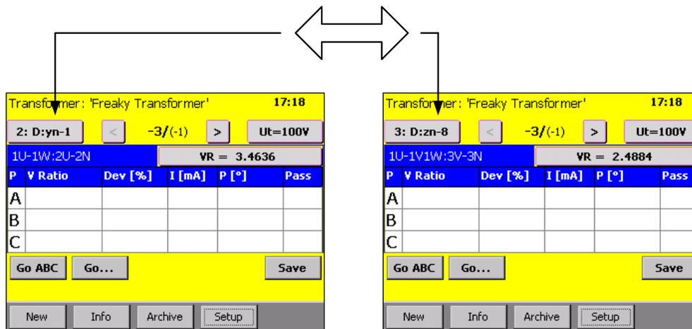
Also take notice of what happens with the tap changer display. As explained in chapter '7.1.5 More Taps', the fixed tap is displayed smaller and in braces, while the free taps appear bigger and bold. As you switch the X-Side from secondary to tertiary, the fixed tap changes also.
