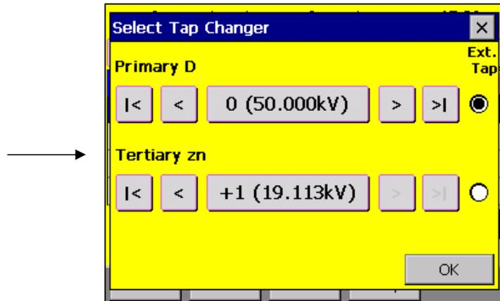
Of course you can too assign tertiary tap changer to be free. Just be aware, that TR-Mk III automatically sets the primary tap changer to be free, when you switch back to secondary winding system on the X-Side.
