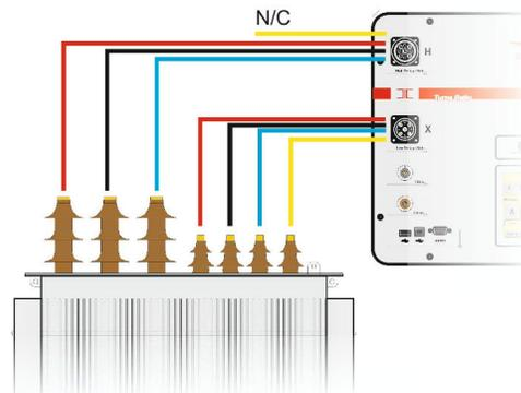
The colored leads are marked to indicate which transformer terminal it must be connected to for correct operation.
