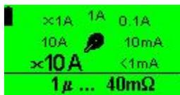
Select the resistance range expected to be measured with the multi-turn Knob. (Selecting the cross current,  $\times 10A$  &  $\times 1A$  measurement range: see page 16). Press the multi-turn Knob when the indicator is pointing at the resistance and current level to be measured (If unsure of current level, then start at the 1 mA range and increase the current range until a valid reading appears).
