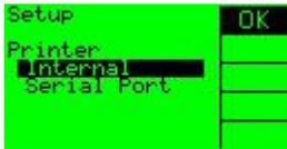
Using the digipot, scroll up or down to select the desired port. After printer or external port is selected, press “OK” to return to the Range Selection Screen.
