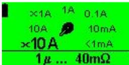
Select the desired test range by turning the rotary knob. The pointer will turn to the available ranges. Press the rotary knob when the desired range is highlighted to select that range.
