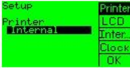
**Internal** – Default for the internal panel mount printer.
