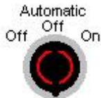
This is the power on switch. Turning the switch to the “ON” position applies power to the test set. Turning the switch to the “OFF” position turns off the instrument. The switch defaults to the “Automatic off” position and will automatically turn off after being idle for a certain period (dependent upon battery charge).
