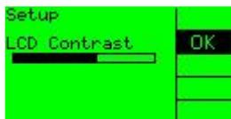
You are now able to adjust the contrast. Using the digipot, turn clockwise or counter-clockwise to adjust the brightness or darkness of the screen.
