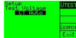
Test Voltage Selector Screen (CT Auto selected)
