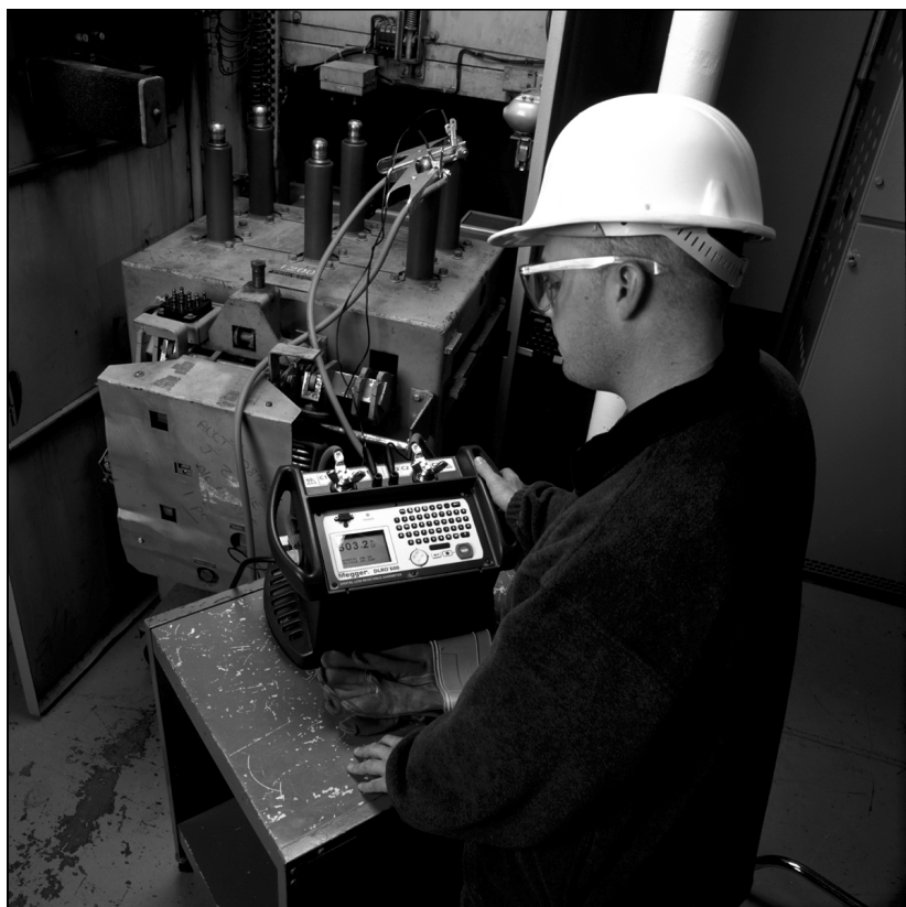
The DLRO600 shown measuring the contact resistance on a GE 15kV air breaker.
