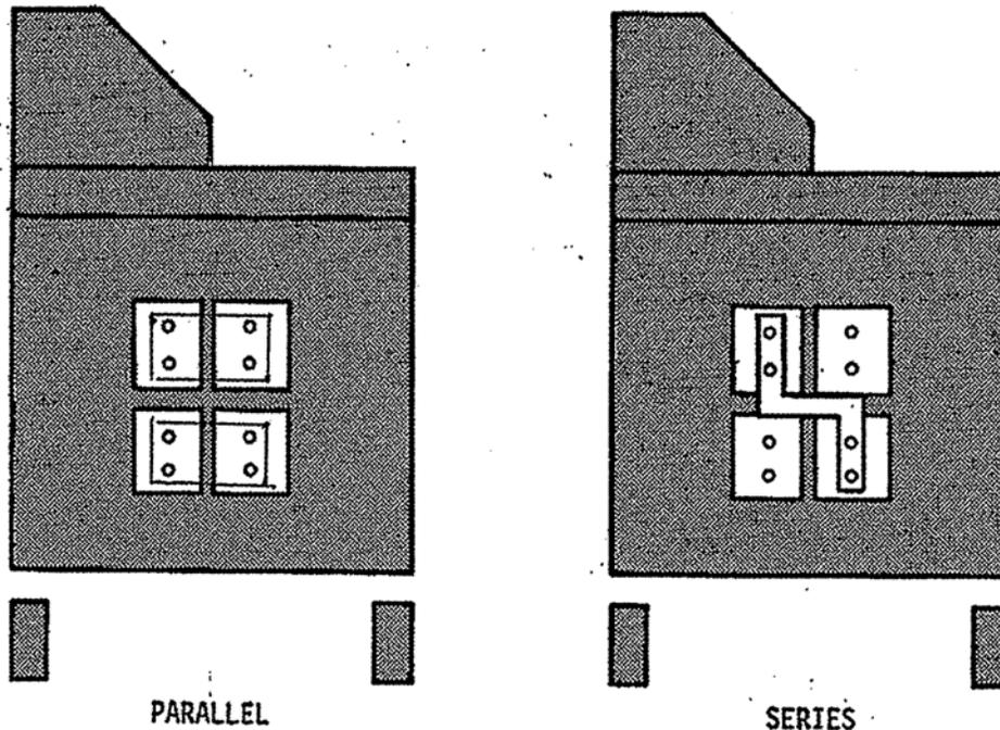
**NOTE:** When the output of the test set is in a series configuration, cabling must be used to connect the output of the test set to the test specimen.
