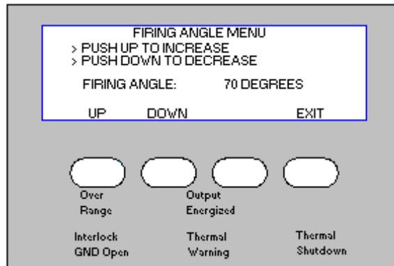
firing angle of the test set, the user can minimize the effect of DC offset and therefore collect more accurate information with regard to the instantaneous characteristics of the test specimen. See ACQUISITION CONTROL MENU for information on how to determine if the output of the test set is symmetrical and how to adjust the firing angle if it is not. The default firing angle is 70°.
