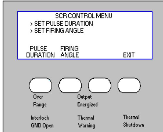
The SCR CONTROL MENU provides the ability to enter into two different areas of SCR adjustment. Pressing the soft key directly beneath PULSE DURATION will display a menu that will allow the user to program the number of cycles that the output of the test set will be energized during a momentary pulse. Pressing the soft key beneath FIRING ANGLE will display a menu that will allow the user to program the angle at which the output signal of the test set is initially energized.
