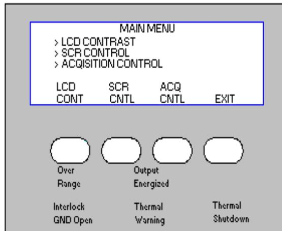
From the MAIN MENU the user may select programming menus to make adjustments to the LCD display contrast, SCR controls, or Acquisition control (current calculation method). The user may also select to EXIT back out to the metering display screen. The desired option would be selected by pressing the soft key directly beneath that option.
