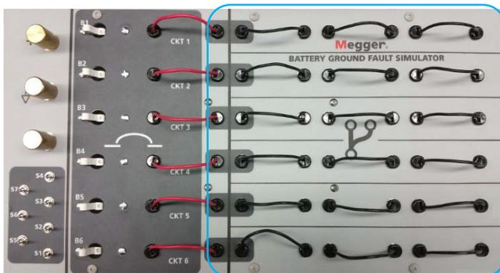
15. Once you have identified where the capacitive phantom faults and the real resistive faults are, turn off breaker 3. (This is never done in the real world.) Now check the fault current from the BGFT transmitter.
