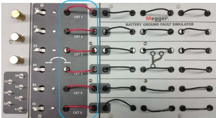
14. Characterize the two circuits using the Wheatstone bridge using the flow chart in appendix A. Locate which one has the resistive fault.
