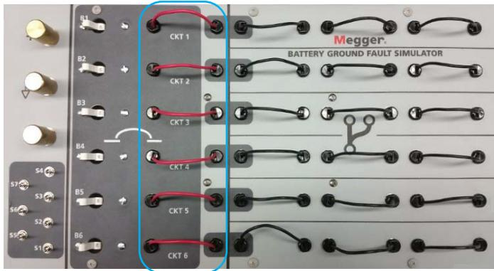
14. Notice that circuit 3 contains both the capacitive phantom fault as well as a resistive fault. You can use the bridge on the secondary side of the circuit to find where the capacitive phantom fault is and where the resistive real fault is.
