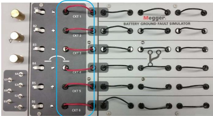
16. Once the faulted circuit is located trace the fault. This is done by moving the receiver's CT down the circuit until the fault current disappears. The point at which the fault current disappears is the location of the fault.
