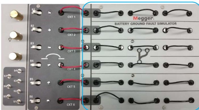
**NOTE:** This is one of the most difficult faults to locate because the impedance of the capacitance of the circuit is lower than the impedance of the fault.
