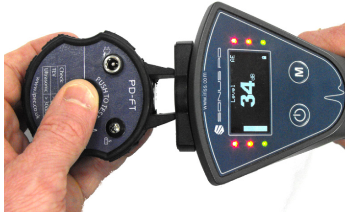
Fig 11: Testing AE function with PD-FT
