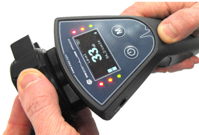
Fig 10: Testing TEV function with PD-FT
