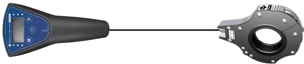
Figure 7: PD Detector connected to the HFCT
