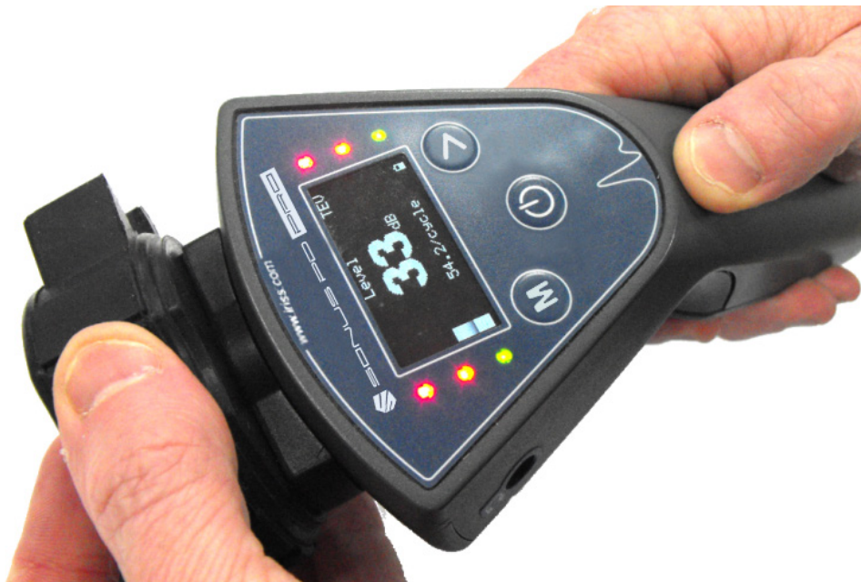
Figure 19: Testing TEV function with PD-FT
