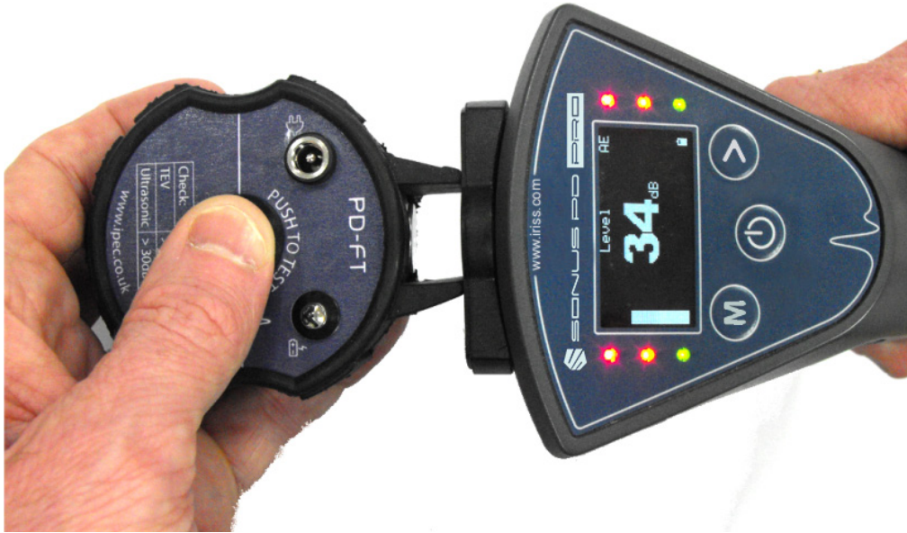
Figure 20: Testing AE function with PD-FT
