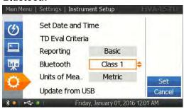
Depending on the Bluetooth setting (Class 1/2/3/Disabled), the device selects the corresponding RF transmission power. Class 1 is the highest; Class 3 is the lowest.
