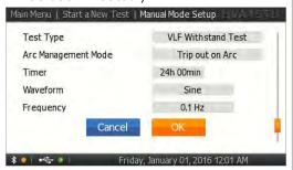
Entering the test voltage before activating the manual mode test by pressing "Start" is optional. In manual mode, the voltage can be set once the test has been initiated!
