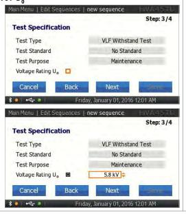
Select this check box if you want to refer to the voltage rating  $\rm U_0$  for definition of the test step voltage. Depending on the DUT type, determine whether to use a three-phase calculation or a one-phase calculation of  $\rm U_0$ .
