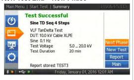
Display indicates end of automatic test.
