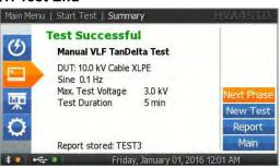
Display indicates end of manual test.
