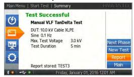
Display indicates end of manual test.
