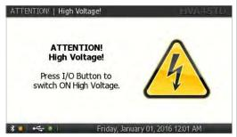
Once the activation screen appears, press the HV switch 40 within 10 seconds.
