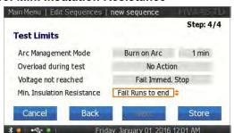
Set action to be taken in case minimum insulation resistance is reached:
