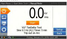
Start the test when the test parameters displayed on the "Manual Test" screen are correct. Rotate the navigation knob until the "Start" field is highlighted. To run the test, push in the knob.
