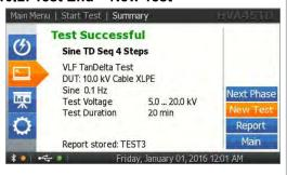
Display indicates end of automatic test.
