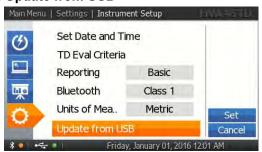
This function is used when installing updates and for transferring information from the PC software to the unit via USB. Insert the USB flash drive before selecting this function.
