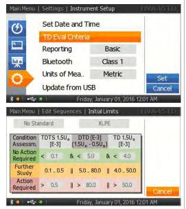
Use these settings to edit default limits for Tan Delta measurements depending on the insulation of the Device Under Test (DUT). These limits are also used for Monitored Withstand Tests (MWT).
