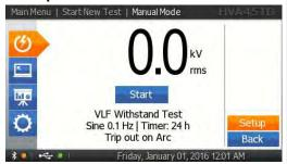
To set the waveform, frequency, or test duration, select "Setup" in the menu. These settings will be remembered for the next test.
