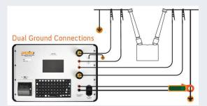
As the rise and fall time is configurable for each test, no transients are induced in the associated apparatus such as current transformers. This avoids maloperation of the connected relays to the current transformers. LRM 200 provides audible signal when test is in progress. LRM 200 provides continuous dc output without overheating. Built in thermal sensor protects LRM 200 overheating if the temperature excess 85° C
