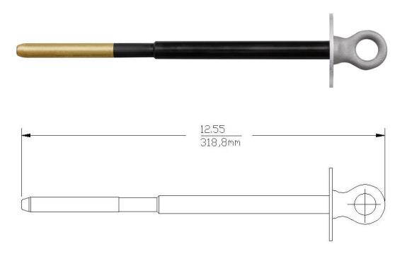
The Elastimold® 370TR test rod is designed to test and allow determination of the condition of the circuit, energized or de-energized. It is designed to mate with all Elastimold® 200 Amp loadbreak bushing products to provide a convenient place to test the circuit with a high voltage meter.
