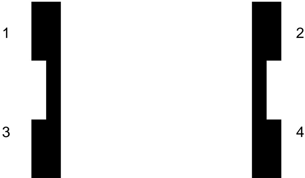
The Stab Adapter Plates connect output terminals 1 and 3 and terminals 2 and 4 together for parallel operation.
