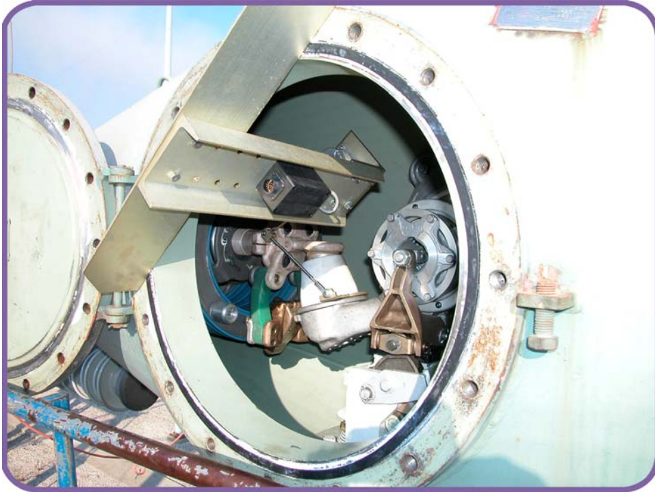
Figure 25. Westinghouse SFA Transducer Installation
