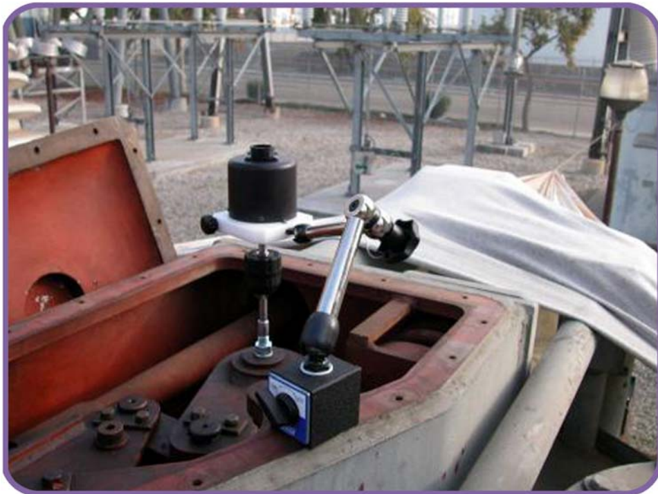
Figure 28. Rotary Transducer on Federal Pacific Breaker
