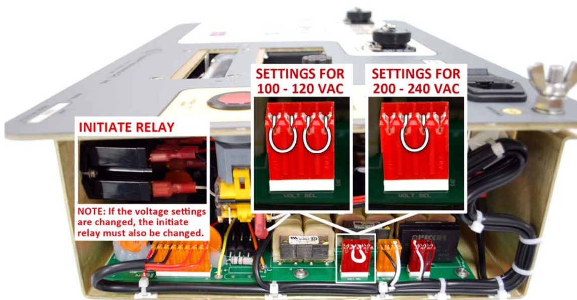
Figure 2. Voltage Selection Jumper Settings and Initiate Relay
