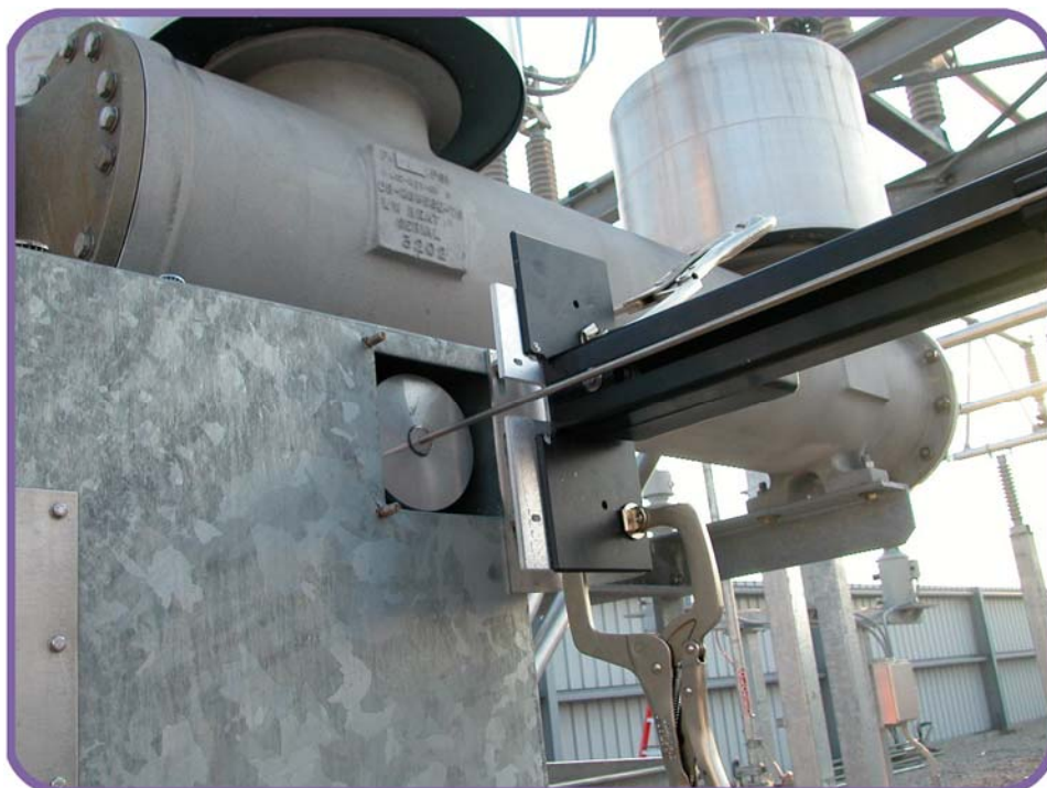
Figure 30. Linear Transducer on Areva DT1-72.5F
