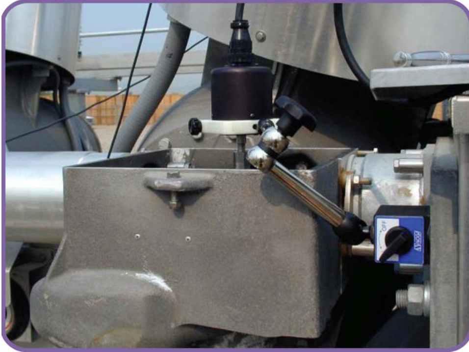
Figure 23. Rotary Transducer on Alstom HE 1014 Circuit Breaker
