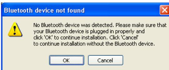
The driver now needs to have the Bluetooth dongle inserted. Plug the dongle into a free USB port. The windows Hardware Installation will now run and some further information windows will appear. Please wait until the Hardware Detection has finished. This screen will then disappear automatically.
