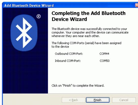
Read the information and note the “outgoing/outbound” COM-Port Number. This number is used by the TD Control Center to communicate with the TD unit.
