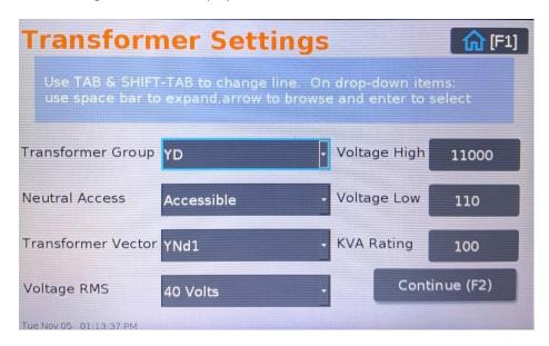
The test parameters can be changed here by pressing the [TAB] key and navigating to the setting that needs to be changed. Press the [F2] key to run the test.
