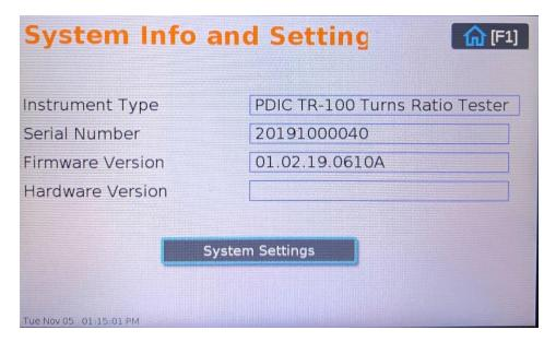
Touch or Press the **[TAB]** key until "System Settings" is highlighted, and then press the **[SPACEBAR]**.
