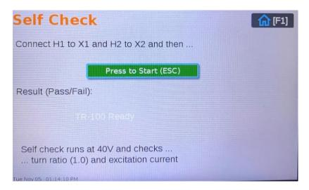
The screen prompts the user to short the H1 cable to the X1 cable and the H2 cable to the X2 cable. Once connected, press the [SPACEBAR]. If the instrument detects a turns ratio of 1, a "Pass" message will be displayed; otherwise, a "Fail" message will be displayed.
