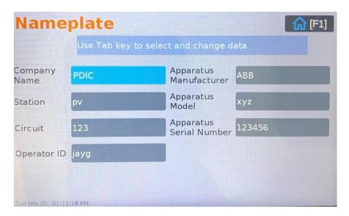
Press the [TAB] key to navigate between the different fields and use the keypad to change the information. Once done, press the [F1] key to return to the Main Menu.
