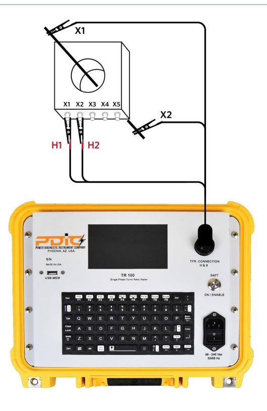
Figure 4: Typical Bushing CT Connection
