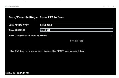
Use the **[TAB]** key to move to the item that you would like to change and press the **[SPACEBAR]**. Make any changes using the keypad and then press the **[F12]** key to save.
