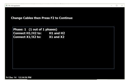
Depending on the type of transformer, the instruments will direct the user to connect the cables accordingly. Once the cables are connected, press the [F2] key to continue the test.
