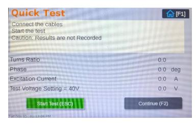
Press the [SPACEBAR] to start and end the test. Once stopped, the test can be re-started by pressing the [SPACEBAR] again.
