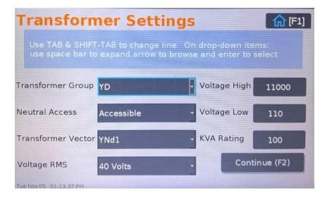
From this screen, first select the transformer type by pressing the [TAB] key to navigate to "Transformer Group" [SPACEBAR] to select either "Single Phase" or "Three Phase".
