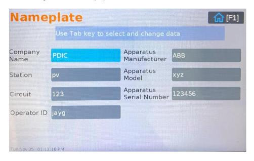
This screen is used to set the apparatus information. Use the [TAB] key to navigate between the fields and use the keypad to make any necessary changes, then press the [F2] key to continue.
