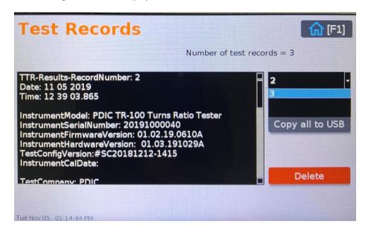
The number of test records will be displayed on this screen. Select the test record from the drop-down menu then press the [TAB] key to select one of the functions on the right. Then press the [SPACEBAR] to execute the selected command. The following commands are available:
