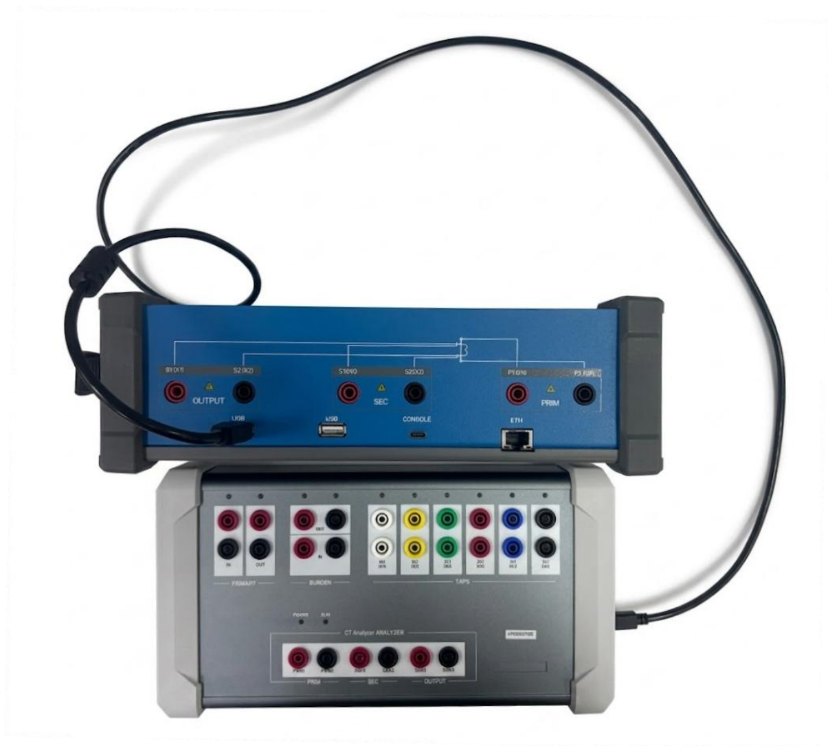
Figure 4-6 USB Connection to Junction Box
